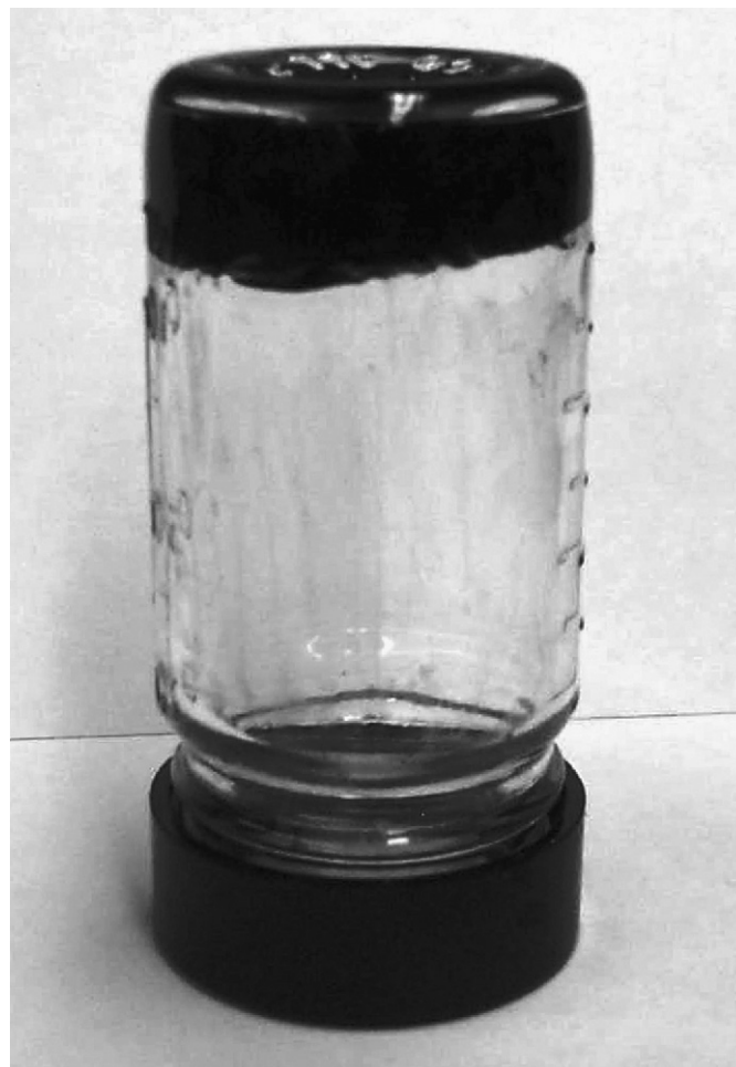
Fig. 8. Photograph of an upside-down vial containing a black gel containing Co nanoparticles and a cross-linked network of oleic acids. In this case, a relatively high concentration of oleic acid (oleic acid/cobalt = 1.3) was used.
